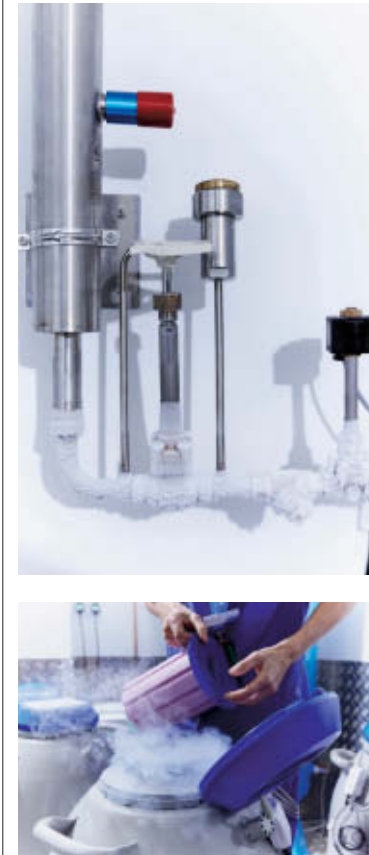
Liquid nitrogen passes through a piping system, top left, before being used to fill storage tanks for the embryos, above left and below, as well as the "baths" in which they are frozen, above right
